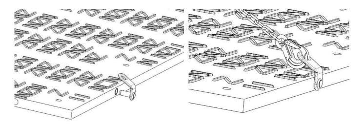
With the help of the chain sling, the panel can be moved to the desired position and installed.
